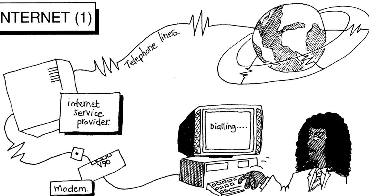
The Internet is a worldwide collection of computers, all linked together by telephone lines. You are charged for using the net but only at the rate of a local telephone call. To get on to the net you will need a computer, a telephone line, a modem and an Internet Service Provider (ISP). You use the modem attached to your computer to connect to a telephone line. You can then dial up the ISP. This is a company which will connect your computer through its own computers to the net.
